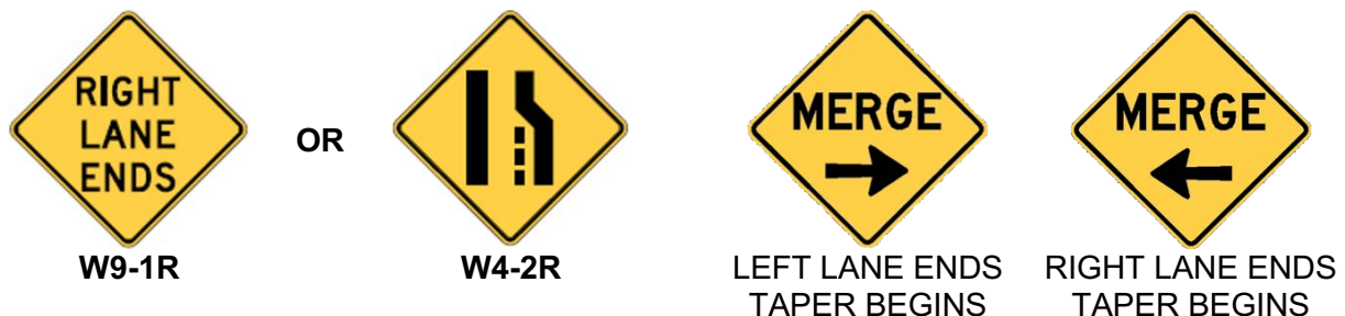
Figure 3. Illustrations of the highest-performing existing signing and the Mn/DOT MERGE with Type A Arrow sign.
